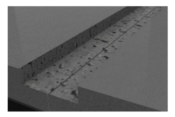
Apply a special primer on all sides of the concrete slab for good adhesion of filling substance. Drill some holes in the concrete bottom positioned at the same distance as the anchorage of the HC-Sinus Slide® repair joint. Install screwed rod trough the anchorage openings and fix into the drilled holes. Level out the HC Sinus Slide® joints down and across.
