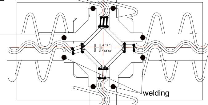
Step 7: Place some additional rebars to reinforce the corners and to prevent uncontrolled concrete cracking at a T-crossing.
